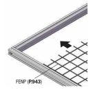
Procedure② Insert a mesh fence into a dedicated slot. The slots may be slightly tight.
