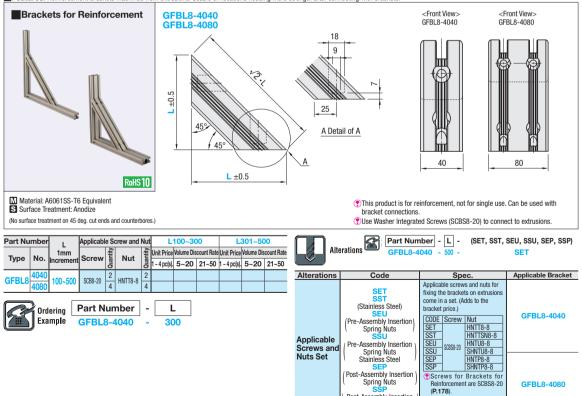
Spring Nuts Stainless Steel Not RoHS compliant when -SET, -SEU or -SEP are specified.
