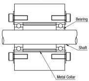
Used to secure bearing.
