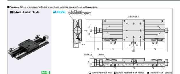
Moment Load Capacity (N·m) Part Number Stage Surface Travel Distance Travel Distance Load Capacity (N) Motion Weight **Unit Price** per Rotation (mm) Parallelism Type (mm) (mm) Horizontal Pitching Yawing Rolling (kg) 80x80 24 128mm 147 25µm 11.5 0.9
