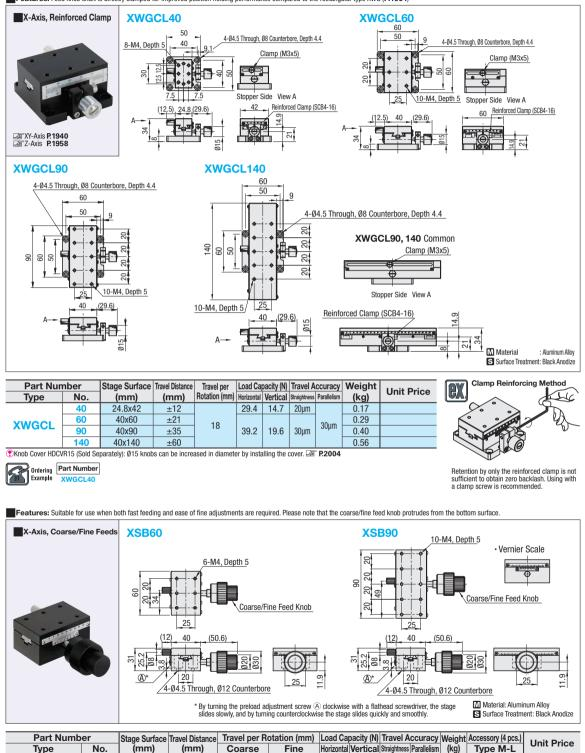
Features: Feed knob shaft is directly clamped for improved position holding performance compared to the rectangular type XWG (P.1904)
