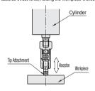
**Features:** Clamps a workpiece from the side by spring force.
