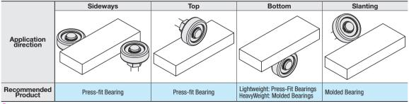
Note that even if it is applied from top, side and bottom, if there is unbalanced load due to mounting accuracy or backlash of work, or when used in high rotation, Urethane of the Press-Fit Bearing may come off.
