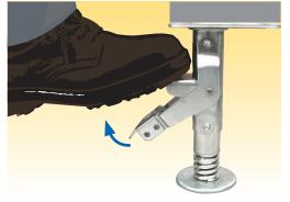
When the Up pedal that went up by locking the truck was stepped, the DOWN pedal goes up. When the DOWN pedal goes up to the point that the pedal touches your foot, release your foot from the pedal slowly. By doing so, the lock can be safely released.
