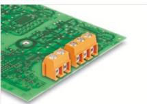
PCB terminal with leaf spring screw connection in 5.00 and 5.08 mm pitches for wire cross-sections up to 2.5 mm<sup>2</sup>.
