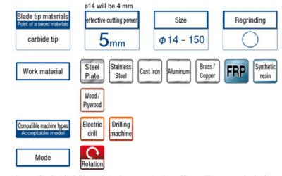
In case the electric drill is used at a degree greater than  $\emptyset 40$ , we will recommend using it at a low speed.
