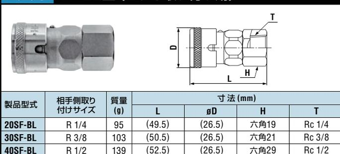
Technical drawing of SF-BL type socket (steel) showing dimensions L, H, T, D, and B.
