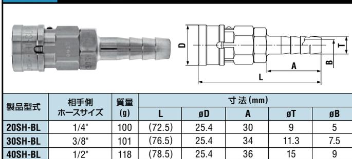
Technical drawing of SH-BL type socket (stainless steel) showing dimensions L, A, B, T, D, and B.
