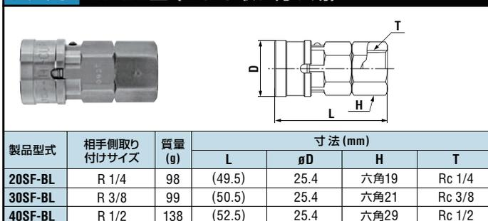
Technical drawing of SF-BL type socket (stainless steel) showing dimensions L, H, T, D, and B.
