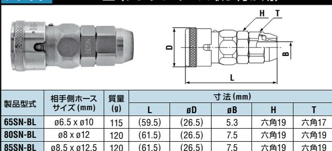
Technical drawing of SN-BL type socket (steel) showing dimensions L, H, T, D, and B.
