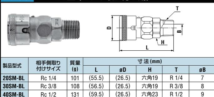
Technical drawing of SM-BL type socket (steel) showing dimensions L, H, T, D, and B.
