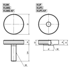
• KUM has a round-shaped thread tip to be distinguished from KUMS KUMS-KF.
