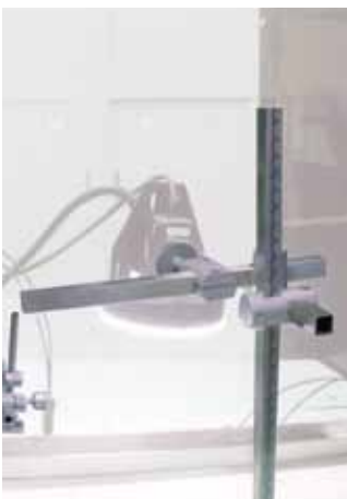
Installation of image lighting equipment with graduated KAKU-pipe
