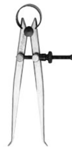
Inside spring calipers
