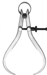
Outside spring calipers
