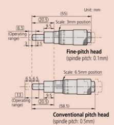
While the fine-pitch micrometer head has a measuring range of 6.5mm, the conventional head has a larger range of 13mm. When replacing a conventional head, the fine-pitch type can use the common range in the middle of the spindle travel. The standard and compact types of fine-pitch head are completely interchangeable.
