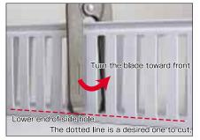
Apply the tip of one blade to the lower end of a side hole. Turn the blade toward front while lightly gripping the handles.
