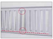
3. The pillar can be cut in line with the lower ends of side holes.
