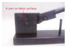
①Remove the screws from the part A on the block surface.
