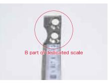
②Align the B part of the exclusive scale with the A part on the block surface from which the screws have been removed.
