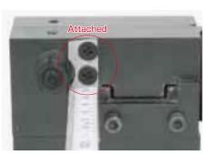
③Secure the B part of the exclusive scale to the A part on the block surface by screws.
