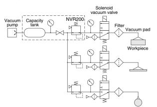
4 Vacuum pressure regulation using vacuum plate
