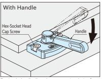
Turning the handle allows the cam to project the jaw for clamping. When the handle is turned back for unclamping, the loaded spring lets the jaw return to the original position.
