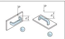
The stated L1 and L2 values denote the average of the breaking loads measured in a drop test with a load of 6.7N.
