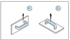
The stated F1 and F2 values denote the average of the breaking loads measured in a breaking test under normal working conditions.
