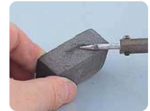
Soldering iron tip cleaning (The soldering iron tip should be cooled before cleaning it.)
